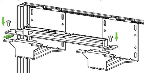
3 Install the actuator all the way up inside the top track on the required side. Adjust the door and fix the actuator with self-tapping screws
