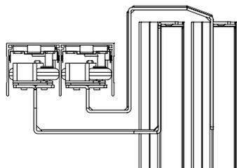
1 Install the optional bracket on the door as shown. Pay attention: the edge of the soft-closer must be in one line with the edge of the bracket.
