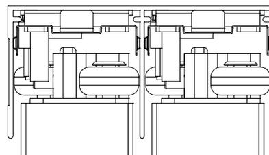
1 Fix the soft-closer with the screws, placing one of the square plates on one side. Install the stopper in one line with the edge of the upper horizontal profile
