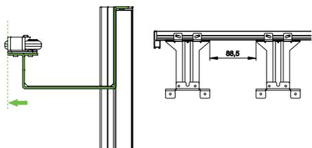
2 Fasten the soft closer to the brackets with screws (included in the kit) with one of the square plates on one side. After that, install the door in the opening or closet. It is not necessary to activate the soft-closer
